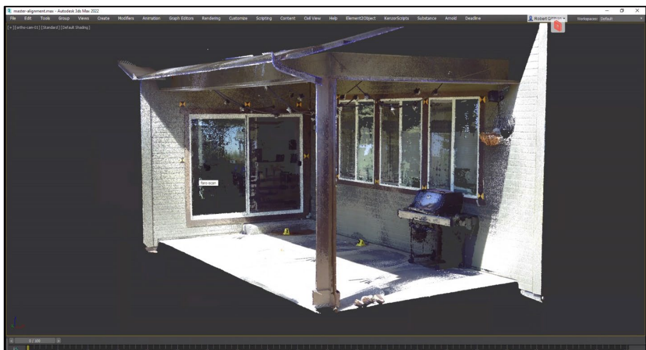
Figure 17. Faro Focus Point Cloud Viewed Within 3DS Max
