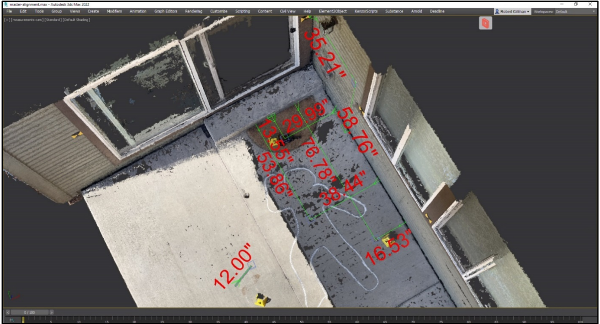
Figure 27. Distance Measurements for the Pix4D Point Cloud
