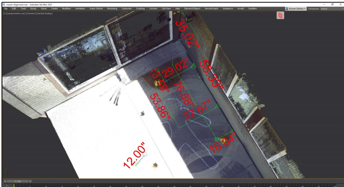
Figure 38. Distance Measurements for the Faro 3D Scanner Point Cloud
