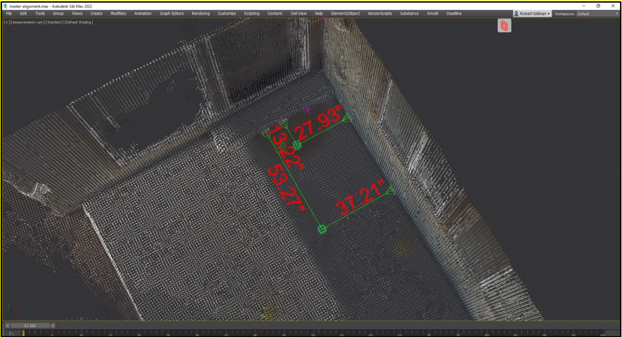
Figure 35. Distance Measurements for the Everypoint Point Cloud
