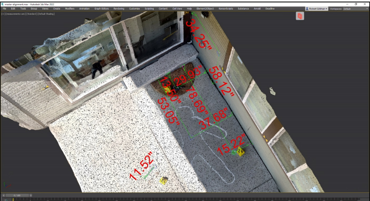
Figure 36. Distance Measurements for the Polycam Point Cloud
