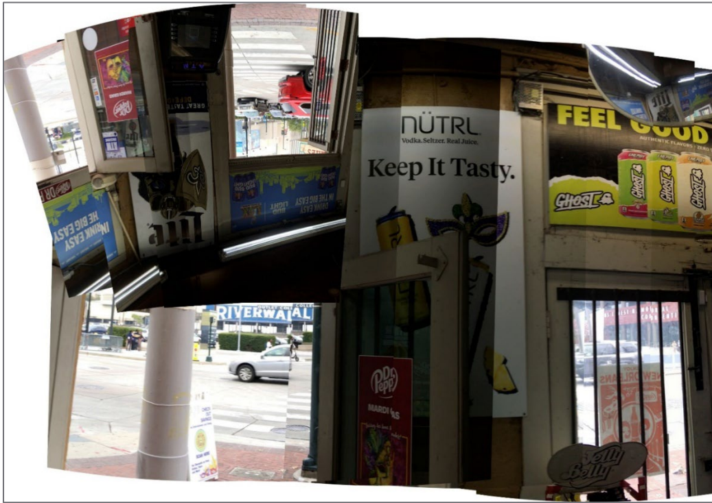
Figure 18. Severe Misalignment Artifact from IMG_0157.MOV (Photoshop Windows)
